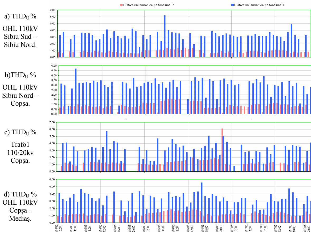
Figure 2 THD U values recorded on OHL110kV Sibiu Sud-Sibiu Nord-Copşa-Mediaş During 15-17 iulie 2006
